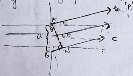
The intensity of central band is maximum & goes on decreasing on both sides.
