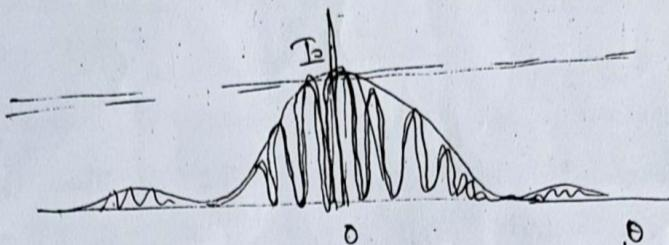
The diagram shows several fringes due to double slit interference, contained in a broad diffraction peak. When the separation b/w the slits is large compared to their width, diff. pattern becomes very flat and we observe only the 2 slit int. pattern.
