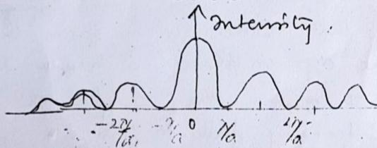
→ Intensity of the central maximum is due to constructive interference of wavelets from all parts of the slit,
