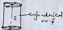
Cylindrical wavefront: When the source of light is linear in shape, like a fine rectangular slit, the wavefront is cylindrical in shape because the locus of all such points which are equidistant from the linear source will be a cylinder.
